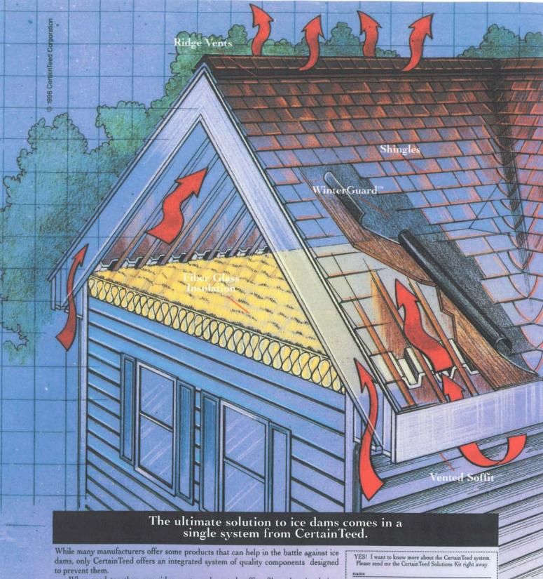
When used together, our ridge vents and vented soffits, fiber glass insulation, WinterGuard™ waterproofing shingle underlayment, and shingles create a roof that's well insulated, properly ventilated and resistant to problems caused by sun, wind, rain, snow and ice.
