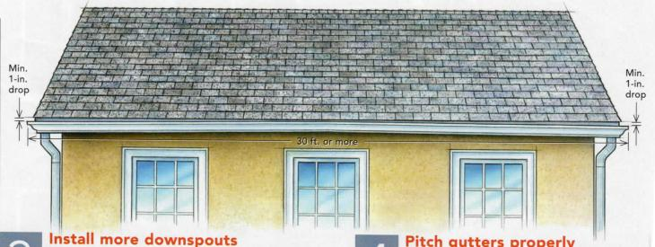
If gutters are longer than 30 ft., pitch them from the middle toward a downspout on each end. The second downspout doubles the capacity of that gutter.
