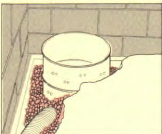
5. Sump well is installed.
