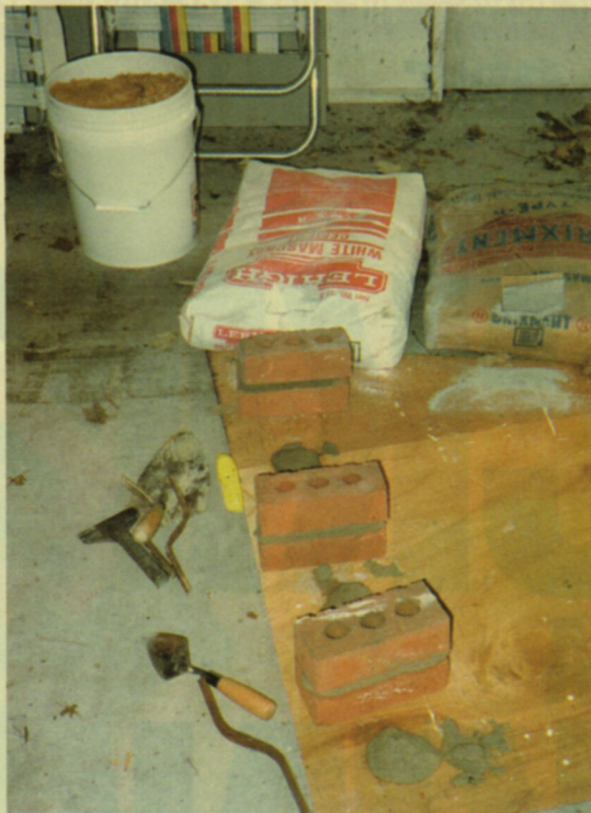
Figure 4. A variety of ingredients make it possible to match existing mortar: white, tan, and gray mortar mixes, black mortar tint to darken the mix if needed, and white and orange sand. Shown in the foreground are some drying samples.
