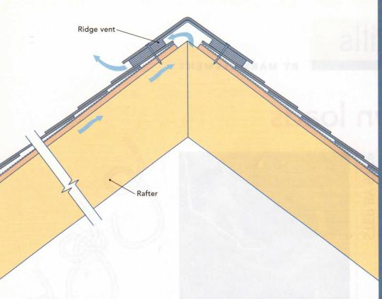
recommends that ventilation channels be at least 2 in. deep, an approach that requires site-built baffles made from thin plywood, stiff cardboard, or rigid foam attached to 2-in. spacers installed in the corners of the rafter bays.
