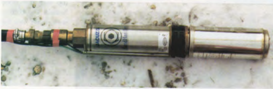
Figure 6. The lower part of the pump houses the motor, and the top half contains the pumping mechanism (the pump head). The plastic section between the two is the inlet for the water. The wires are secured to prevent chafing.
