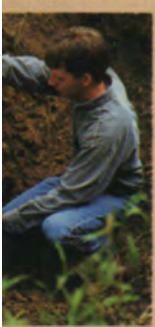
A FEW WEEKS LATER , the excavation contractor got to work. In a matter of minutes, he dug a room-size hole for the new septic tank. INSET: As the first step in any septic system design, the soil at the proposed site must be evaluated. Here, a soil scientist analyzes a test pit. By observing the various layers and matching the dirt to a color-coded key, he is able to determine the type of soil, how well it drains, and the location of the seasonal high-water mark, which establishes the limit of a leach field's depth.
