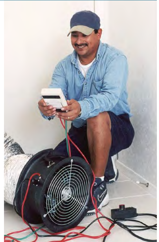
Your contractor may test duct leakage as part of the home's energy audit.
