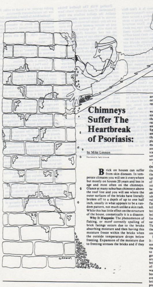
are stressed often enough, the outer layer or face of the brick will separate from the rest of the brick.
